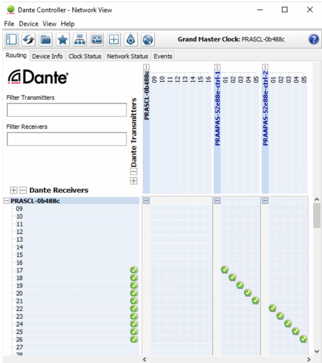
**Figure 5.3:** Routing example for PRAESENSA and PRA-APAS system
